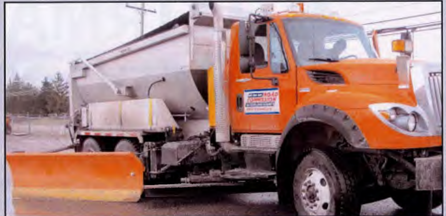
An RCOC plow truck equipped with the new wing plow.
